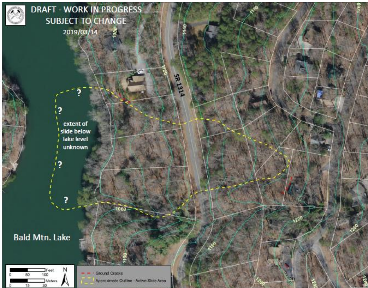
Map showing the approximate area of active slide movement as of 2014/03/14. Topographic contours (20 foot contour interval) derived from a 20-foot pixel resolution LiDAR (Light Detecting And Ranging) digital elevation model. LiDAR data acquisition pre-dates recent slide movement. Parcel boundaries courtesy of the Rutherford County GIS Department. Map base is 2015 orthophotography. Data Sources: North Carolina Geological Survey and North Carolina Dept. of Transportation. Note: All locations and boundaries are approximate. Areas of ground cracks within the active slide area are not shown. This map is not a substitute for a map prepared by a licensed land surveyor.
